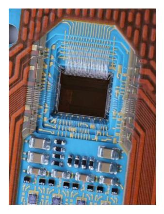
*Figure 4: Application 2 – sensor chip - placed in LTCC cavity*
